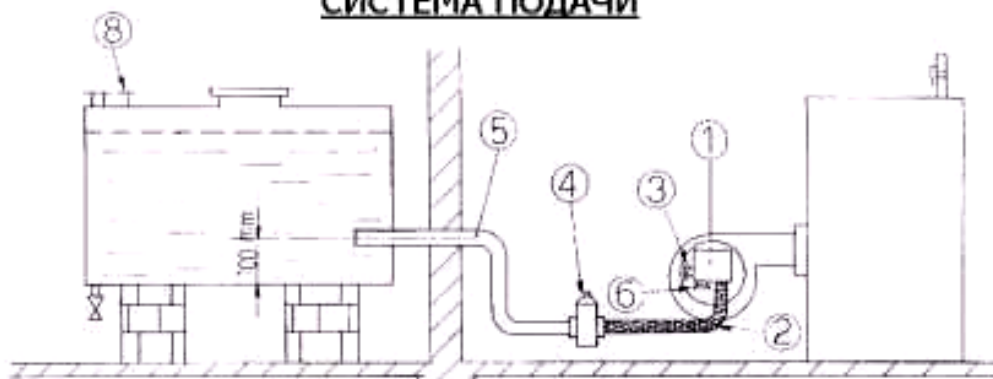
Gravity feeding System with siphon
